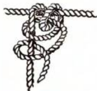
For tying second rope to waist-loop.
